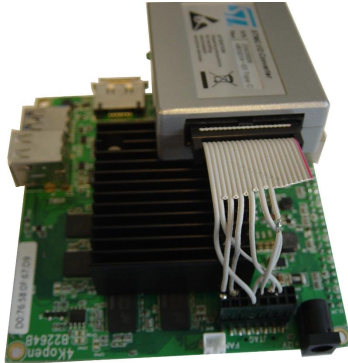
Figure 6 : Example of wiring with flat cable
